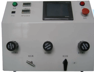
卫星管路多余物自动吹除控制台 Automatic Blow-off Control Console of Satellite Pipeline Contaminant
