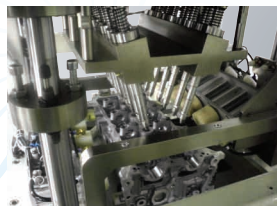
提升气缸-凸轮轴-导杆-气门拍打-进排气门封堵 Cylinder lifting-camshaft-guide rod-valve flap-intake & exhaust valve plugging
