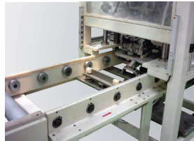
无动力滚筒-自动识别位置 Gravity roller-automatic identification of position
